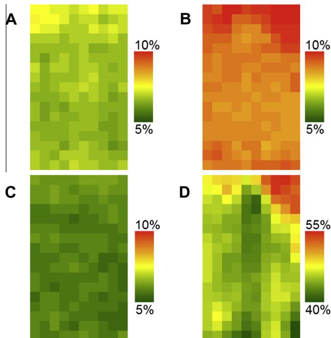
**Fig. 4.** Spatial variability of the surface spectral reflectance for blue (A), green (B), red (C) and near infrared (D) bands over green grass. (For interpretation of the references to color in this figure legend, the reader is referred to the web version of this article.)
